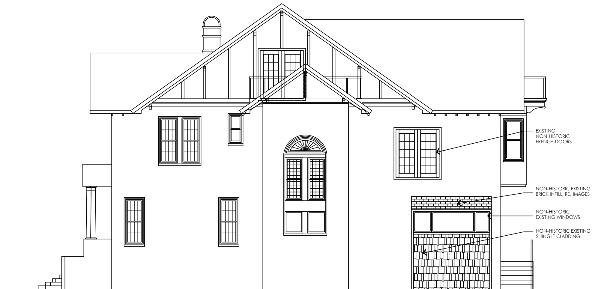
EXISTING NORTH ELEVATION
