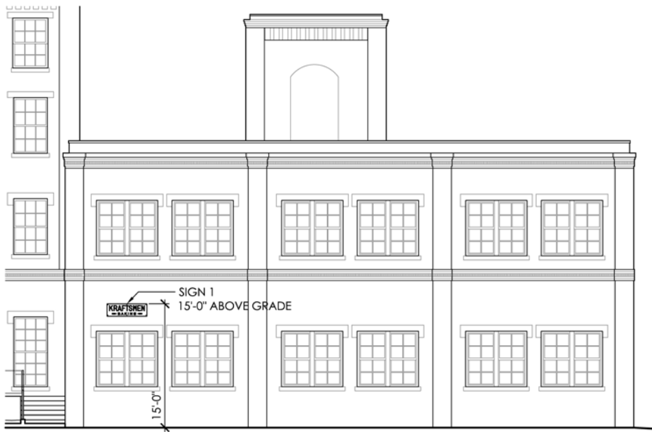
2 SOUTH BUILDING ELEVATION 1/16" = 1' - 0"
