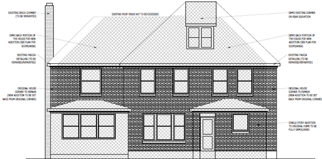
2 EAST ELEVATION - EXISTING 1/4" = 1'-0"
