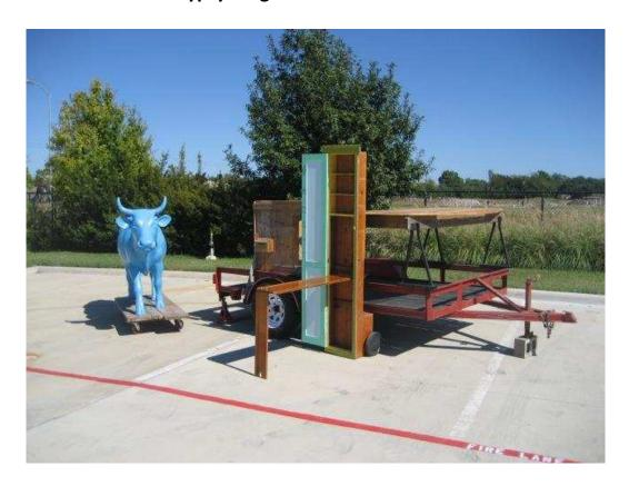
Over the past three years, I have been collecting a number of reused items so that I could build a "wagon". The results of my efforts are The Gypsy Wagon. An 8' x 10' trailer had been sitting in a nearby lot, with rotted floorboards, tires, and electrical wiring. I talked with the owner and made an easy agreement to take the trailer. New tires, wheels, lights and tags and the foundation was done. (Not a good idea to use recycled tires, wheels, or electrical wiring!)
