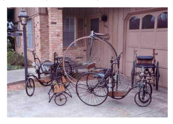
To properly restore antique vehicles one is obliged to use recycled materials as a necessity. The bicycle, three tricycles, and trailer required restoration. The 1889 55" Columbia Light Roadster required parts but not the diversity as the tricycles.
