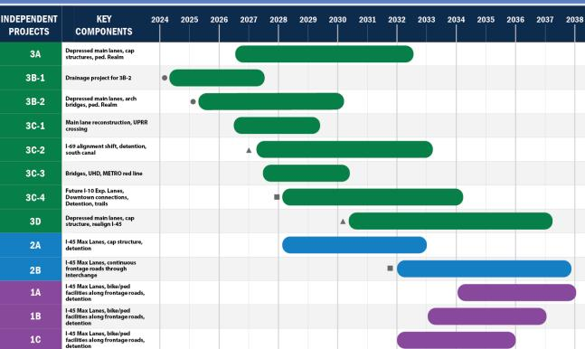
3B-1 is phased to start before 3B-2 because drainage elements in 3B-1 need to be constructed and operational to receive drainage from 3B-2.
