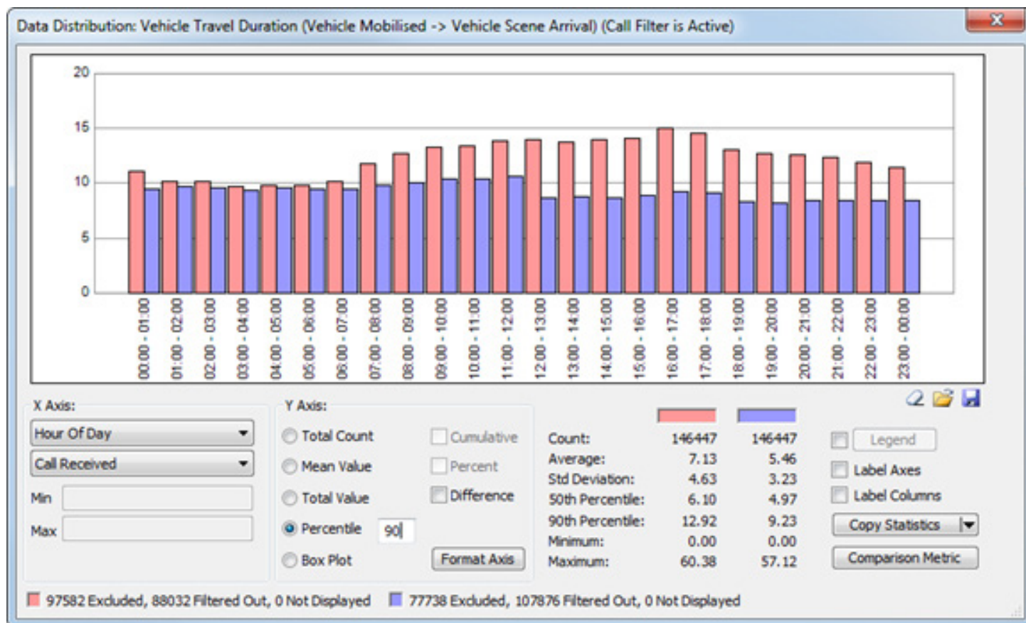
Figure 39 – 90th Percentile Travel Time for Transport Vehicles by Time of Day (pink) simulated baseline, (blue) simulated with additional 70 peak-time ambulances
