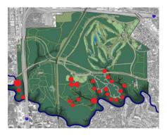
Erosion Coincides with Steep Slopes and Concentrated Water
