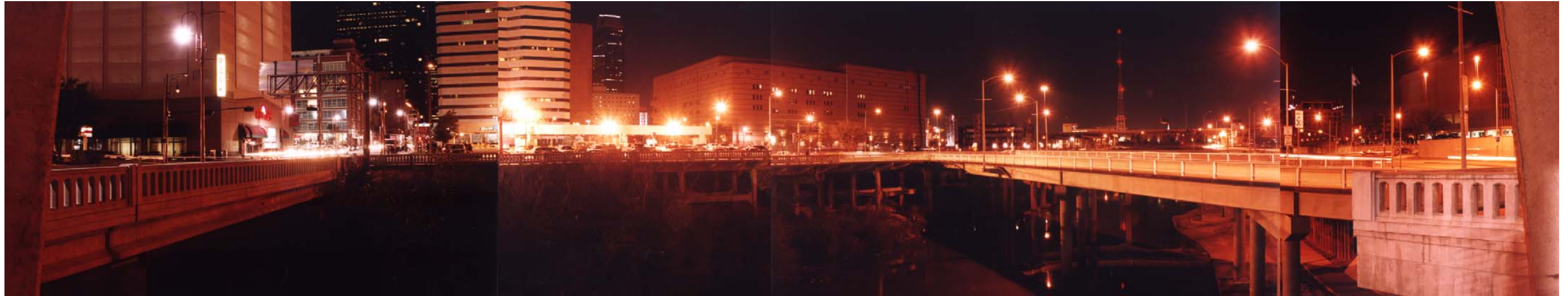
Existing street lighting produces glare and spill into the unlighted bayou.
