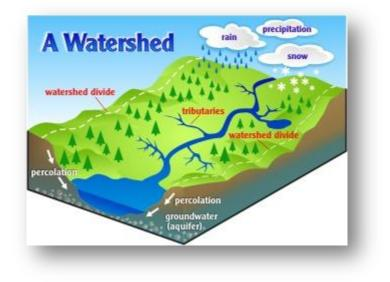
Figure 1 – Diagram of a watershed
