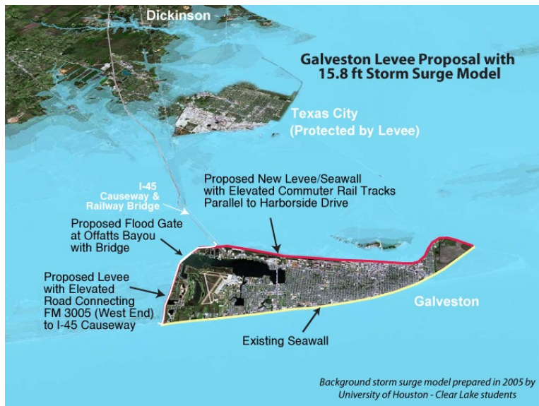
Figure 1. Proposed Galveston Levee system and existing Texas City levee shown with 15.8-foot storm surge and the resulting flood protection. Potential additional benefits of the plan to other developments for Galveston Island are also indicated. The exact course and components of the system would be determined by a detailed feasibility and engineering study. The community recommends that this study be initiated immediately.
