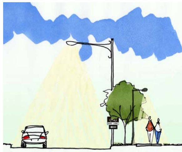
Street lights at COH standard 200' spacing. Pedestrian lights at 60' spacing along sidewalks
