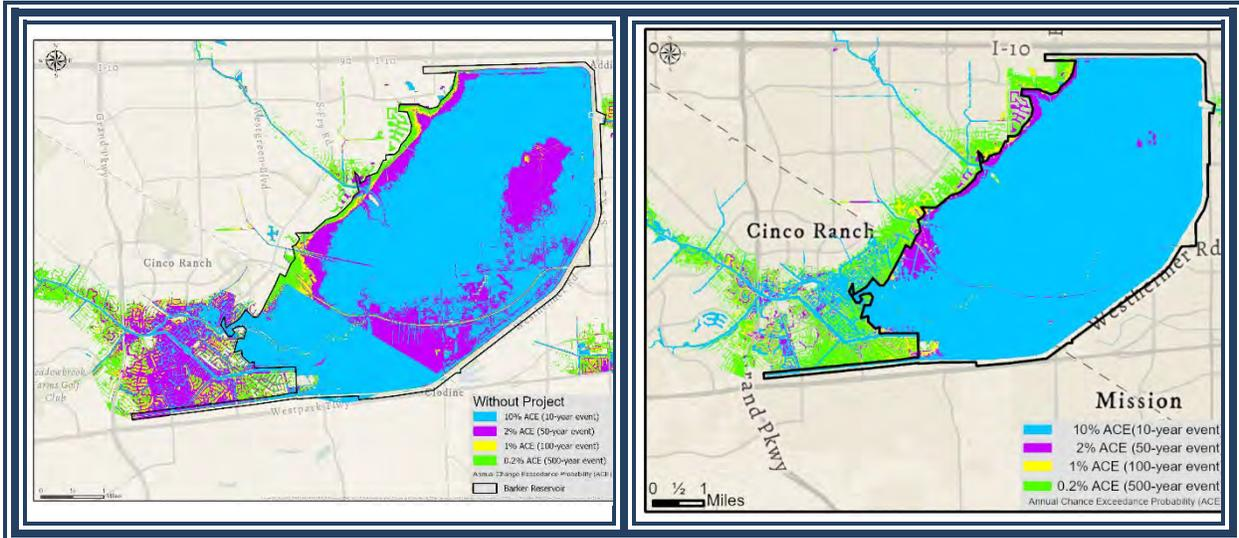
**Figure 23. Barker Reservoir Maps Showing Existing vs. Future Without-Project Conditions**
