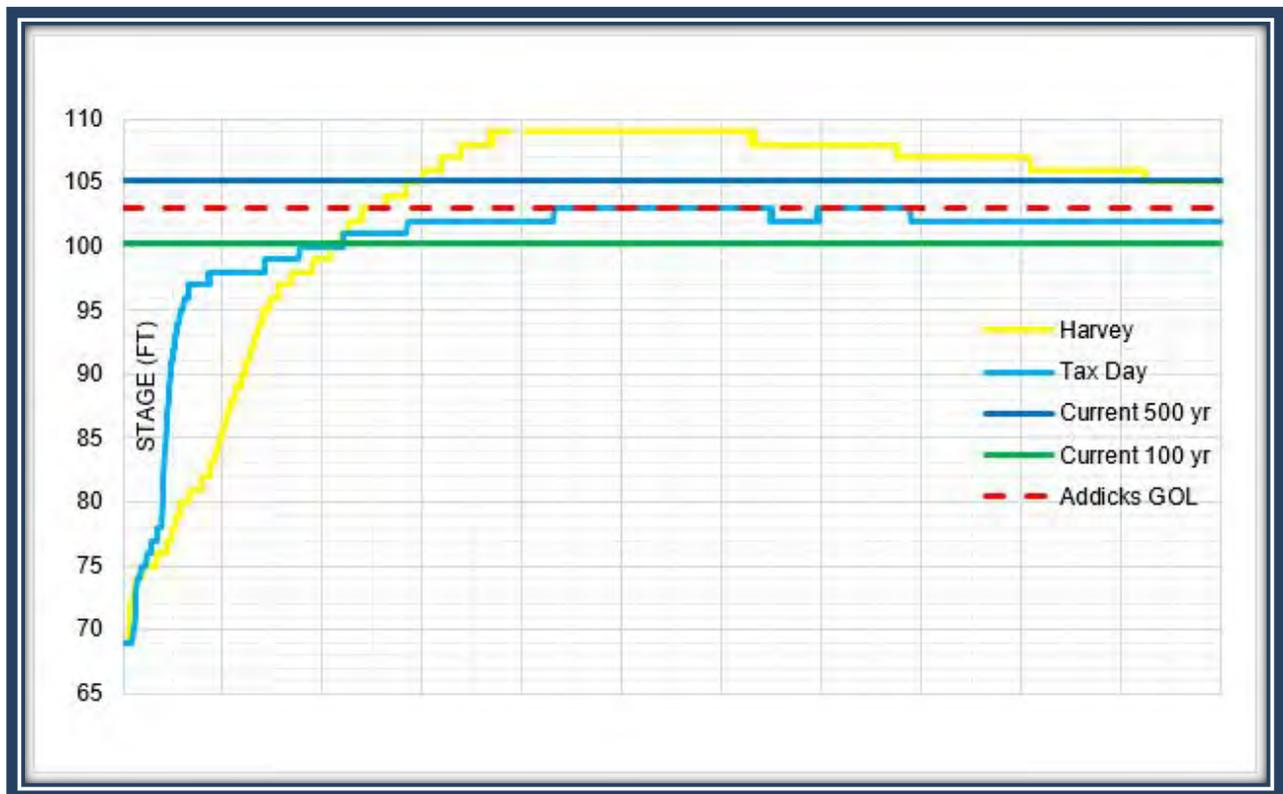
**Figure 1. Observed Elevation of Hurricane Harvey at Addicks Dam**
