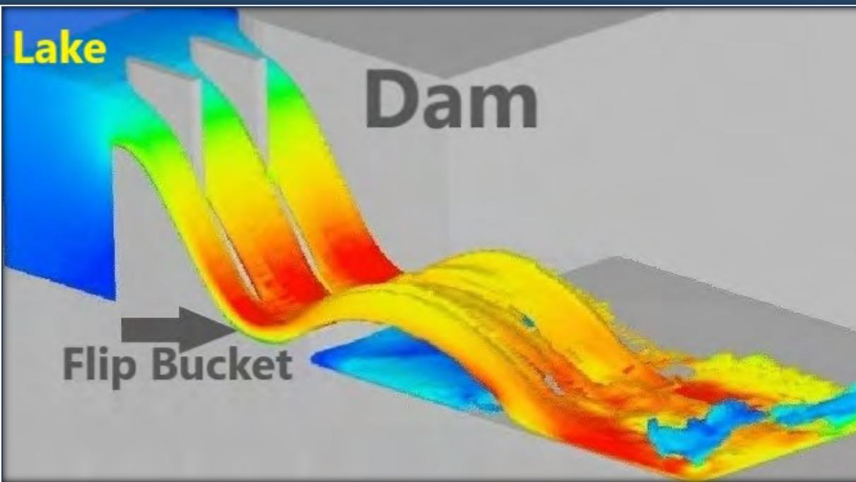
Figure 73. Typical Flip Bucket Configuration Showing Water Energy (Red = High Energy, Blue = Low Energy)
