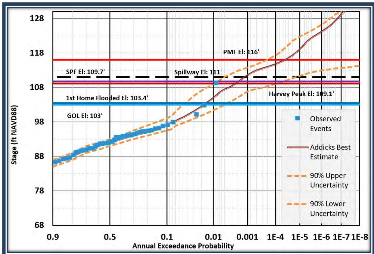
Figure 51. Addicks Pool Frequency Curve (USACE 2020)
