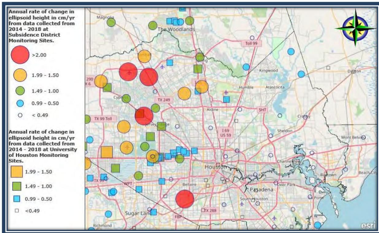
Figure 19. Subsidence Rates in Harris and Surrounding Counties in Centimeters per Year (0.394 cm = 1 inch)
