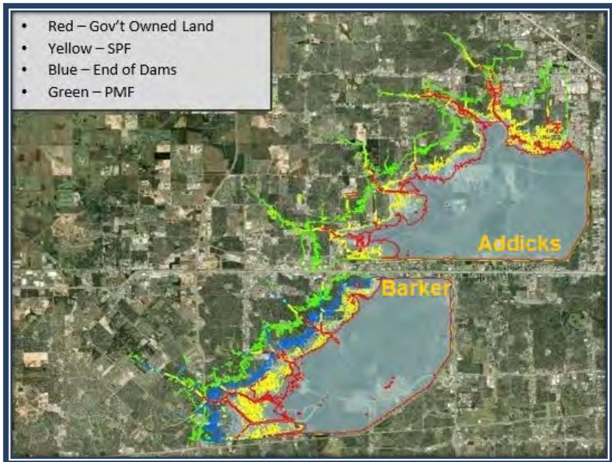
**Figure 5. Map Showing Various Elevations at Addicks and Barker Reservoirs**
