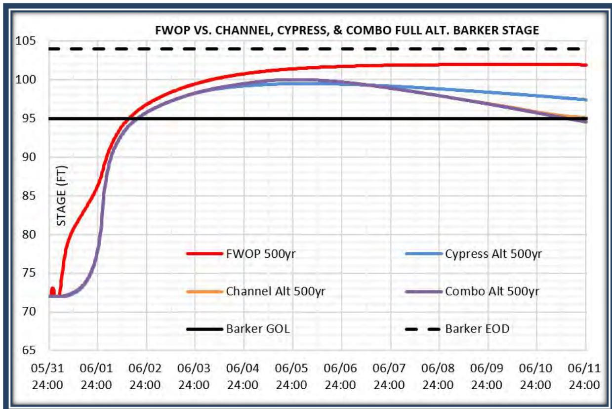
Figure 4. Barker Reservoir FWOP 0.002 AEP vs Alternative Plans 2, 6, and 8
