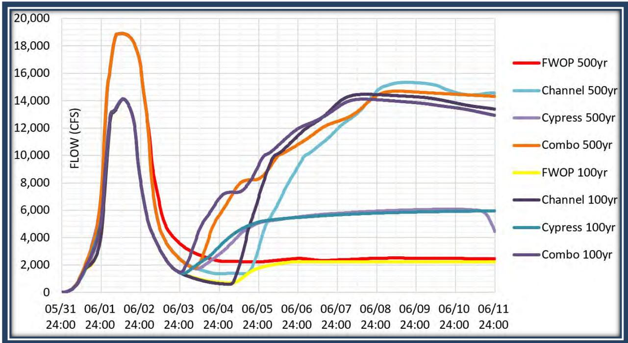
**Figure 65. FWOP and Alternatives Flow at Barker at Piney Point**
