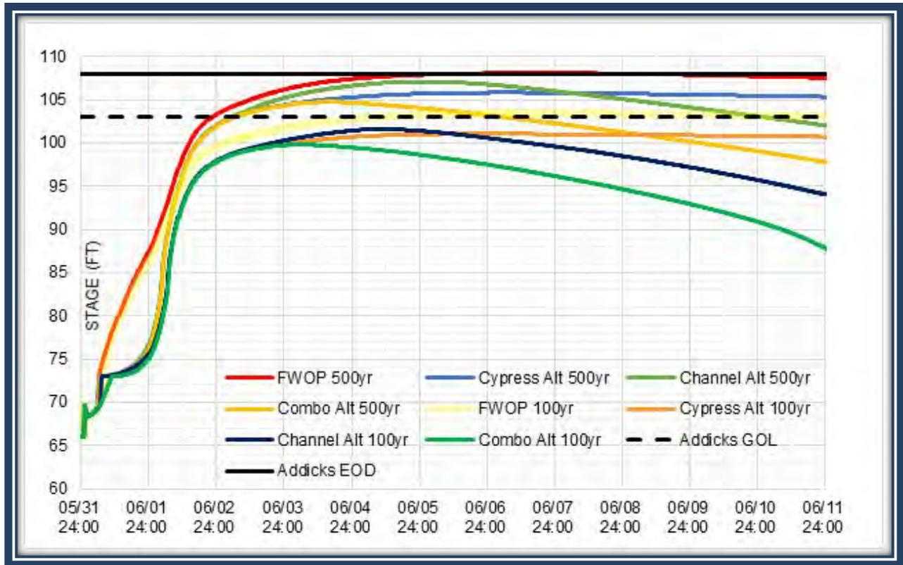
**Figure 59. Addicks 500-Year Stages for FWOP and Structural Alternatives**
