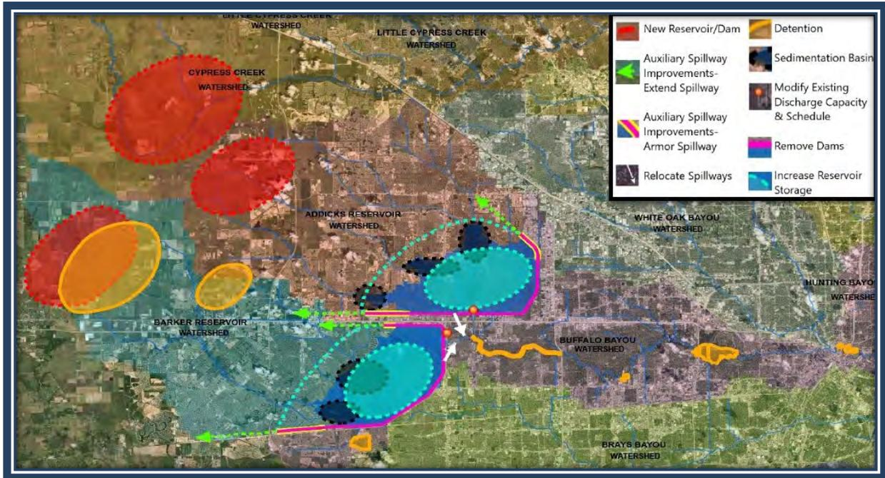
Figure 28. Structural Measures to Increase Storage within the System
