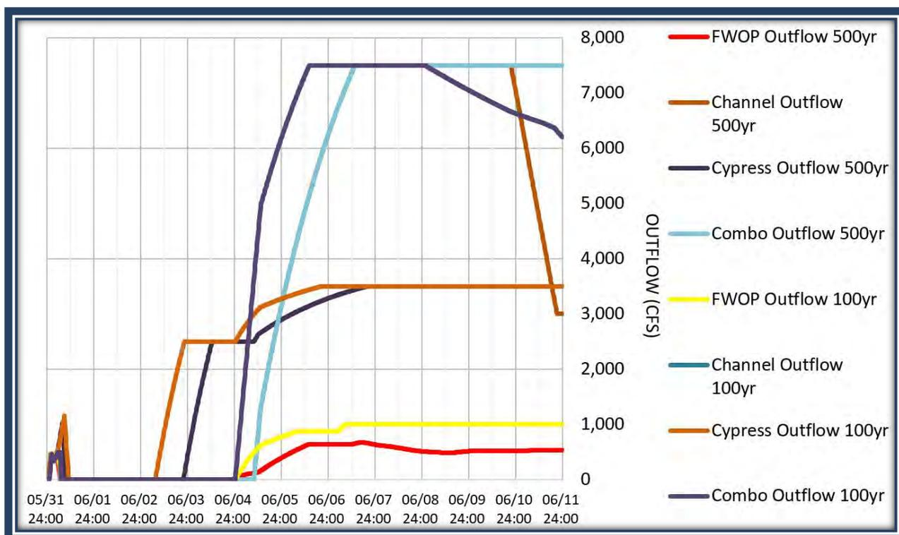
Figure 64. FWOP and Alternatives Outflows at Barker
