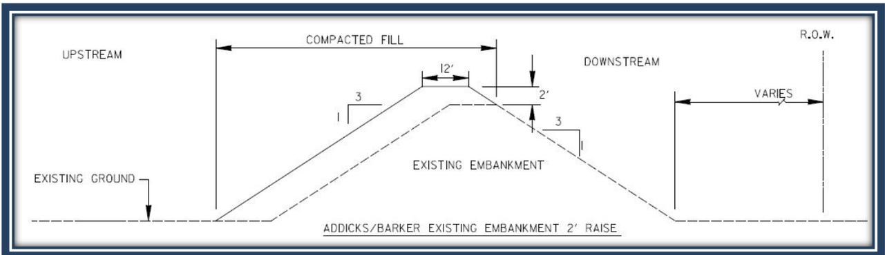
Figure 39. Typical Embankment Raise
