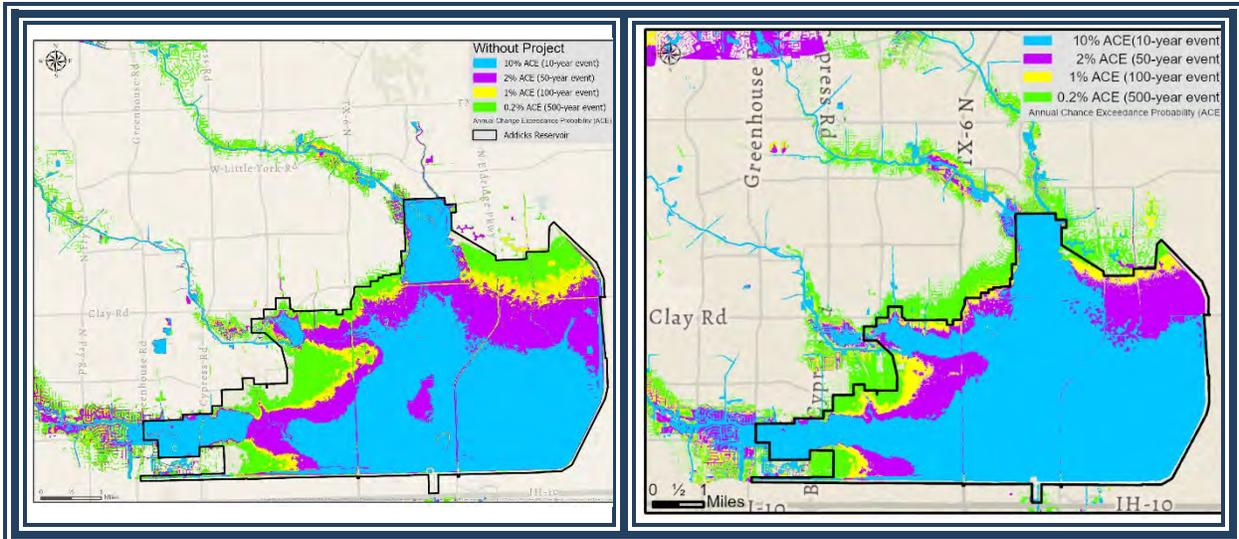
**Figure 22. Addicks Reservoir Maps Showing Existing vs. Future Without-Project Conditions**
