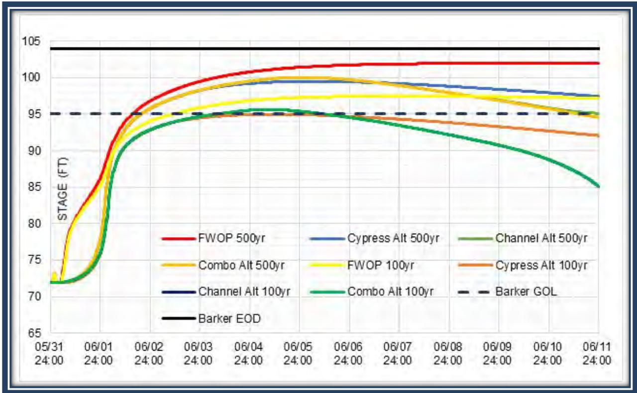
**Figure 60. Barker 500-Year Stages for FWOP and Structural Alternatives**
