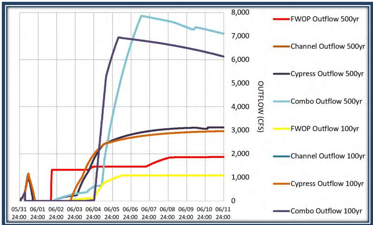
**Figure 63. FWOP and Alternatives Outflows at Addicks**
